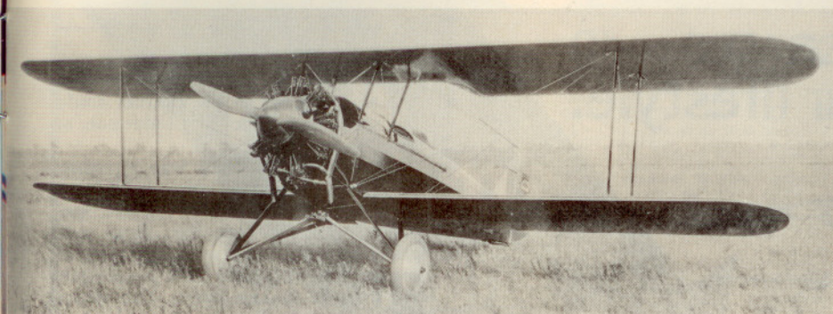
The 1926-27 Laird LC, with 200-hp Wright J-4 Whirlwind engine, wide-track landing gear, and such refinements as lights and parachute flares for night flying. This was an early use of a steel spring leaf as a tailskid.
